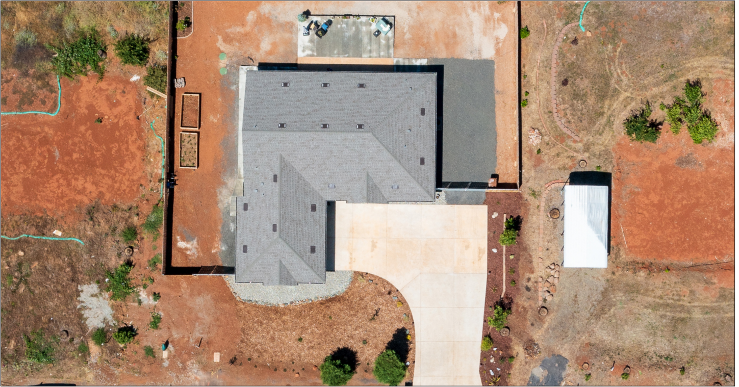
Zone 0: Example of a house employing a noncombustible 5-foot area immediately surrounding the home.
